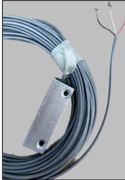
Figure 17. Magnetic Limit Switch wires
